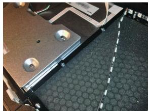
Place the magnet backed, inner light strip section back to the inner light frame wall, making sure the LCD mounting screws go between the magnet strips on the back of the light strip. Now it is time to
