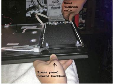
These bottom 2 mounting points also secure the speaker panel's hinges. The hinge mounting points are mounting SLOTS and not mounting HOLES. So you need to make sure you are pressing the speaker panel all the way toward the backbox when they are tightened down. If you do not do this and the panel has shifted, it will cause the speaker panel to not close properly.
