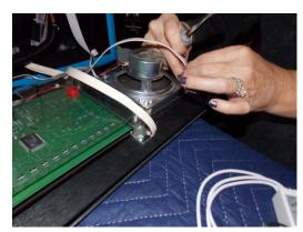
4B. (Upgraded Speakers)Place the LED Light frame on top of the grill making sure that the screw holes are (DOWN) and that the lead wire coming off is near the bottom corner of your DMD. Once in position, replace the speaker and screw in all 4 corners using the extra long screws. Remember to hook the ground strap back on.
