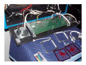
2. Remove your speakers and speaker grill to prepare for installation of the light kit. Nuts removed will not be re-used.
