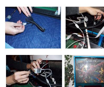
9. Lift the playfield, locate the power cable and pull it along the right side of the cabinet up to the auxiliary power plug. Plug it up and you're finished. Close up the machine and try it out.
