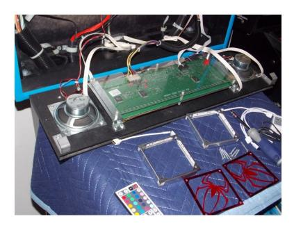
2. Remove your speakers and speaker grill to prepare for installation of the light kit.
