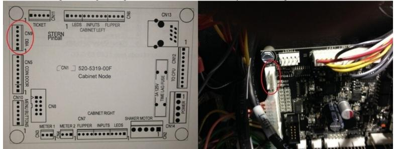
Locate Cabinet Node 1 in your SPIKE System game. This is a printed circuit board that is located inside the coin door on the left side of the cabinet (inside the cabinet, below the left flipper button). On **Cabinet Node 1** you will find the **CN9** connection on the top left area of the board.
