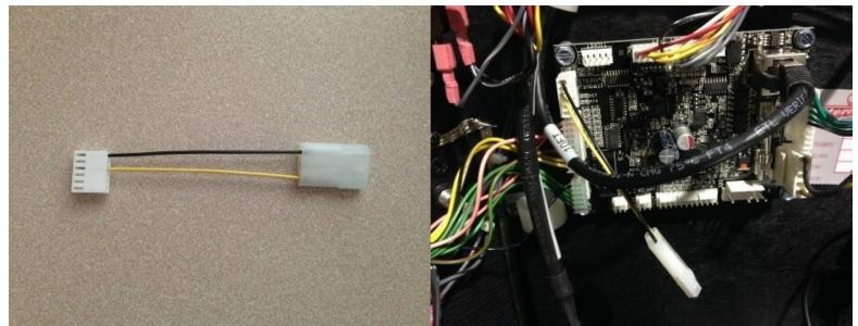
Plug the SAM to SPIKE 12v Power Harness into the CN9 connection. This harness connection is keyed so it can only be plugged in the proper direction.
