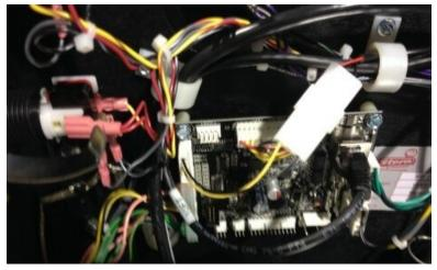
Plug the 2 pin end of the power cable into the SAM to SPIKE 12v Power Harness. Route the power cable through the cable clamps, along with the other wires, and into the backbox where it will plug into the RGB controller.
