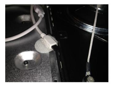
The RGB output wires and light strip connection cables can then be looped in a way to take up a bit of their slack and they can be taped down on the back of the LCD screen to secure them. Each of the 2 light strip connection cables need to be plugged in the 4 holed RGB controller output wires. These connections each have an arrow on the end of the wires. The wires should be plugged in together so the ARROWS LINE UP WITH EACH OTHER.
