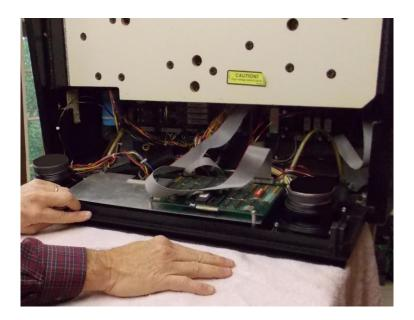
1. Power down system, pull the translight, and remove speaker panel.
