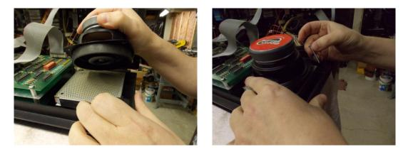
5. Once in position, replace the speaker and screw in all 4 corners using the longer screws. Remember to hook the ground strap back on.
