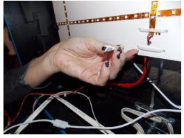
8A. (Stock Power Supply Install) Locate the power cable and plug into the LED controller. Next run it up to the power board and attach the alligator clips to the correct test points. The power board is the one located at the upper left side inside the head/backbox. Make sure to clip Red onto +12V and Black onto the GROUND
