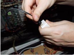
b. Locate the 6 pin power connector on your Sound board and unplug it. (See picture Below)
