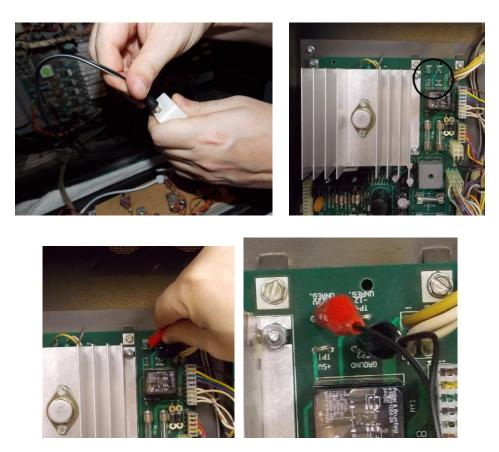
8B. (Aftermarket Power Supply or Stock Power Supply Install) Addition power adaptor is required and can be purchased separately from the Data East / Sega light kit page at \_\_\_\_\_\_ if you didn't choose to include it with your kit. This install is required if you have an aftermarket power supply or if you find that your test points are broken or missing from your stock power supply.
