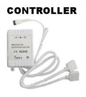
7. The controller has a sensor eye. Make sure that wherever you decide locate/mount the controller in the backbox that the eye is above the level of the speaker panel and behind the translight. It will work fine through the translight. TIP: use Velcro to mount the box in your desired position.
