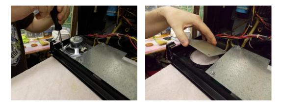
3. Next place your speaker light kit into position making sure that the screw holes are down against the panel and that the lead wire coming off is near the bottom corner of your DMD, followed by the grill.
