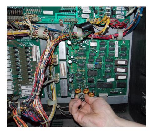
b. Insert the power splitter end of the power cable as seen below and re-attach your original cable to the splitter secondary connector.
