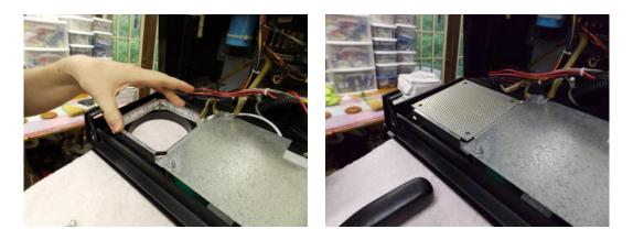
4A.(Stock Speakers) Once in position, replace the speaker and screw in all 4 corners using the longer provided screws with the kit. Remember to hook the ground strap back on. (IF YOU HAVE UPGRADED SPEAKERS INSTALLED SEE NEXT PAGE)
