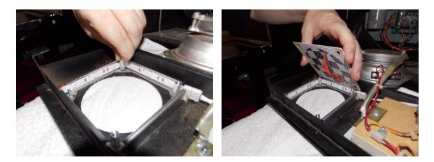
5A. (Stock Speakers) Once in position, replace the speaker and screw in all 4 corners using the provided screws with the kit. Remember to hook the ground strap back on. (IF YOU HAVE UPGRADED SPEAKERS INSTALLED SEE NEXT PAGE)
