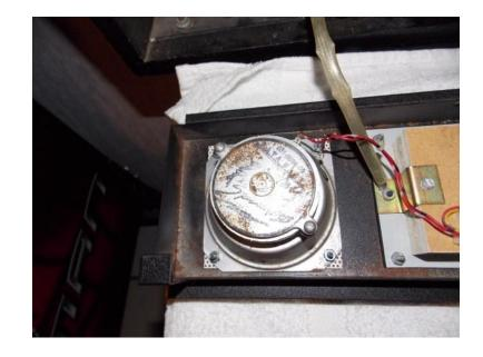
1. Power down system, pull the translight, and remove speaker panel.
