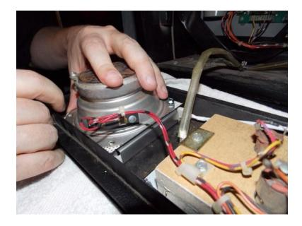
5B. (Upgraded Speakers) Will work, but you will need to locate longer screws at your local hardware store. It is impossible for us to accurately assess the correct sizes needed for all of the different variety of Data East / Sega machines. You will need to evaluate your panel and locate the correct size needed from your local hardware store. They should be common sizes.
