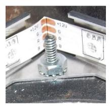
4. Install 4 hex spacers (Provided) as follows. Thread each spacer down till they touch the nut. Then, put the speaker grill back in place and install the speaker. See speaker install options in the next 2 steps for both (stock) and (upgraded) speakers.
