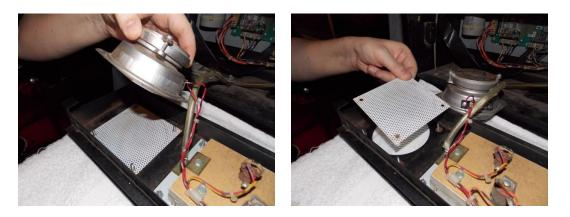
3. Next place your speaker light kit into position and set it down onto the existing threads sticking up from the panel and make sure that the lead wire coming off is near the bottom corner of your display. Use the nuts you removed in the previous step to secure the plate.
